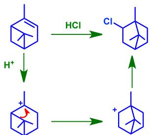
Relief in strain from four to five membered ring is driving force
