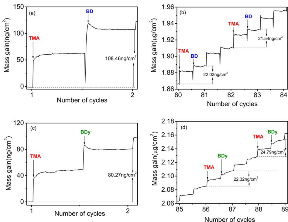
Fig. 5. (Color online) Mass gain measured by *in situ* QCM during (a) first TMA-BD cycle, (b) linear growth regime of TMA-BD, (c) first TMA-BDy cycle, and (d) linear growth regime of TMA-BDy.
