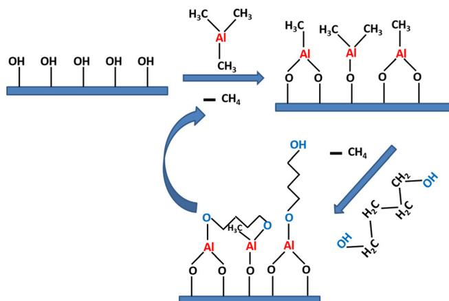
FIG. 8. (Color online) Probable reaction mechanism of alucone film growth using TMA and BD considering a 2:1 stoichiometry.
