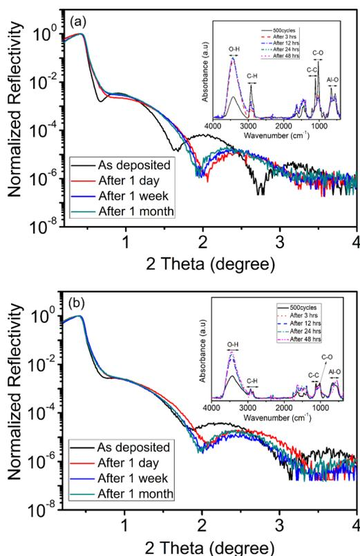
Fig. 10. (Color online) Comparison of thickness and chemical nature of (a) TMA-BD and (b) TMA-BDy alucone films on continuous exposure to the ambient as measured by XRR.
