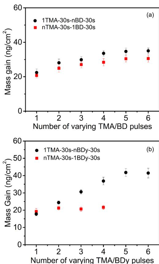
FIG. 3. (Color online) Self-limiting behavior of (a) TMA and BD precursors and (b) TMA and BDy precursors measured using *in situ* QCM during alucone deposition.
