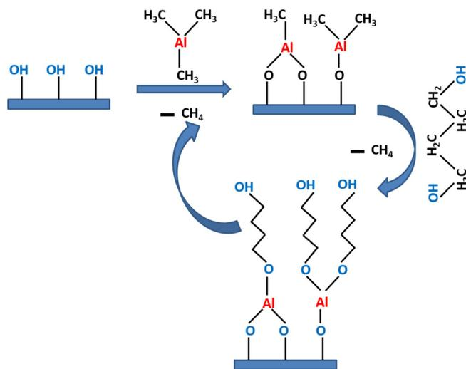
Fig. 1. (Color online) Probable reaction mechanism of alucone film growth using TMA and BD considering a 2:3 stoichiometry.
