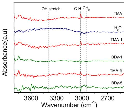
Fig. 6. (Color online) *In situ* FTIR spectra of the last TMA-H<sub>2</sub>O cycle and the first and fifth TMA-BDy cycles.
