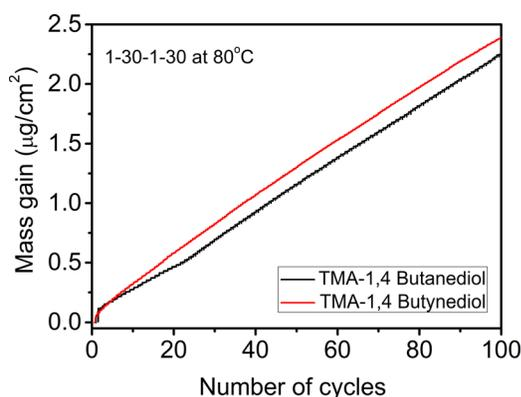
FIG. 4. (Color online) Linear growth for 100 cycles of alucone films deposited at  $80^\circ\text{C}$ .
