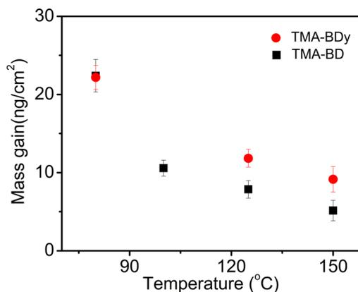
Fig. 2. (Color online) Mass gain vs deposition temperature for TMA-BD and TMA-BDy as measured by *in situ* QCM.
