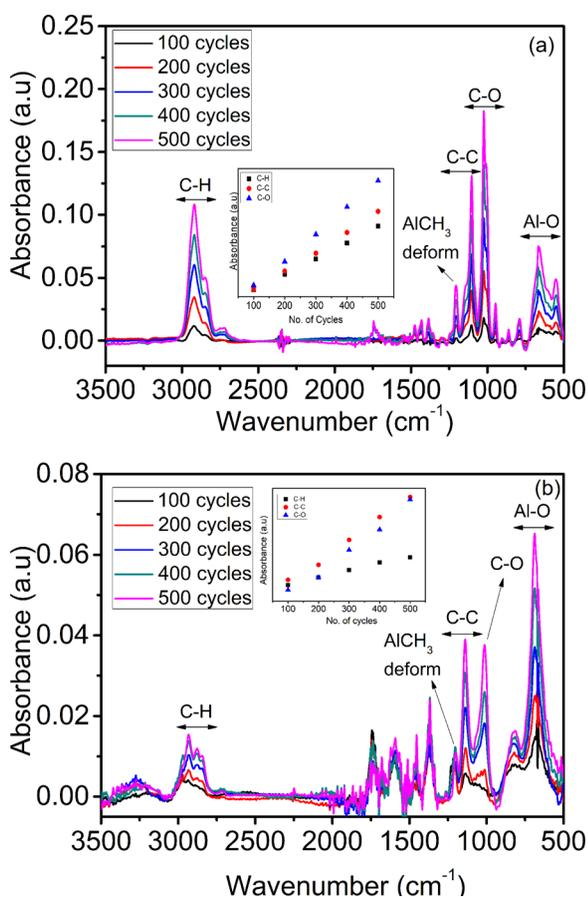
Fig. 7. (Color online) Vibrational spectra of (a) TMA-BD and (b) TMA-BDy with an increase in the number of deposition cycles.
